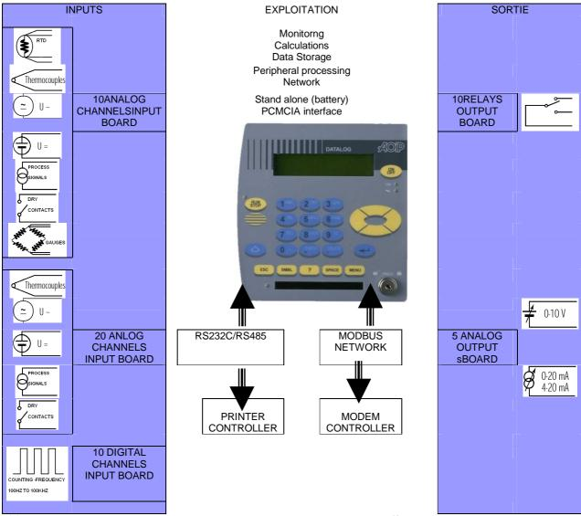
(1)Full, half- or quarter- bridge gauges. Need a power supply board which occupies 1 I/O slot. (2) RS 485 or RS 232C network interface. MODBUS/RTU (binary) protocol. Up to 32 modules can be linked. D < 1 200 m.
